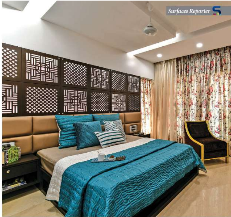
A backlit customised hand board comprises of laser cut panel with classical geometric motifs
